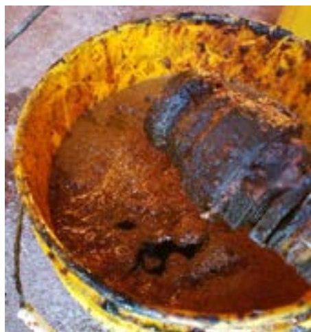
Figure 11. Example of sediment collected from an oil storage tank. (Source: J. Lechman, J&R Consultants, Ltd., Winnipeg, MB, Canada).
